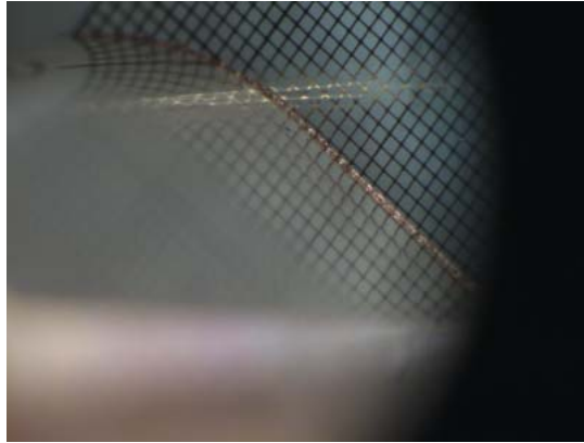
Fig. 19 Evaluation of size of cornice-type burrs on R2mm ridge with 0.1mm mesh pattern.
